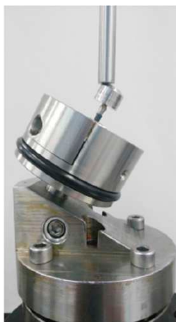
Figure 2. Clamp of the fatigue test machine.
