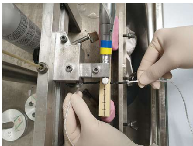
Fig. 2 Specially designed device for measuring changes in temperature during implant osteotomies
